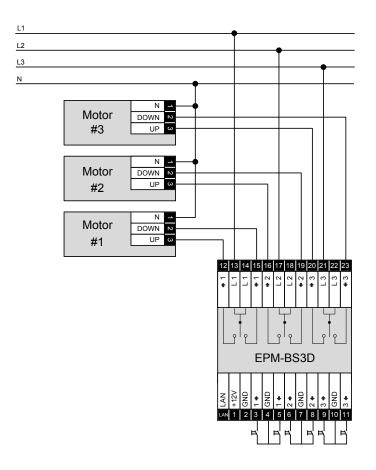
The Highcross EPM-BS3D module can be used with high-voltage (220V AC) and low-voltage (12-48V DC) motors. The L terminals of every group can be connected to different types of power, according to properties of used motor.
